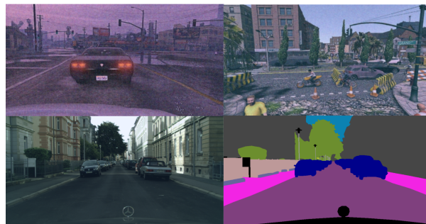
Figure 17: Textured textured images from GTA5 and Synthia (top), an unchanged map image from Cityscapes and the respective segmentation map (bottom).
